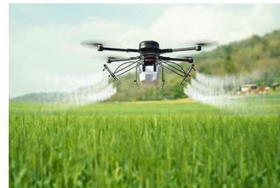
Figure 6. Drift potential from drones with a boom may be excessive depending on the size of the boom and the type and size of nozzle used. Photo by Adobe Stock.
