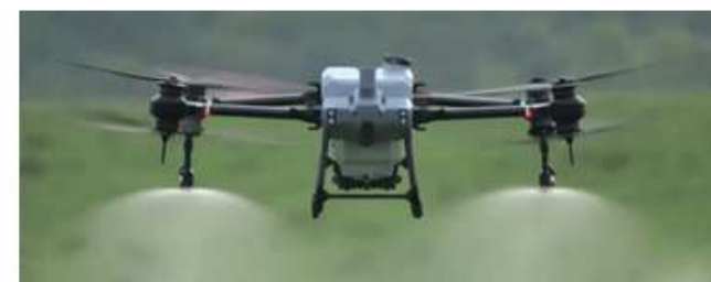
Figure 8a. Spray pattern produced by the dual rotating-disc type spray atomizer. Photo by DJI.com.
